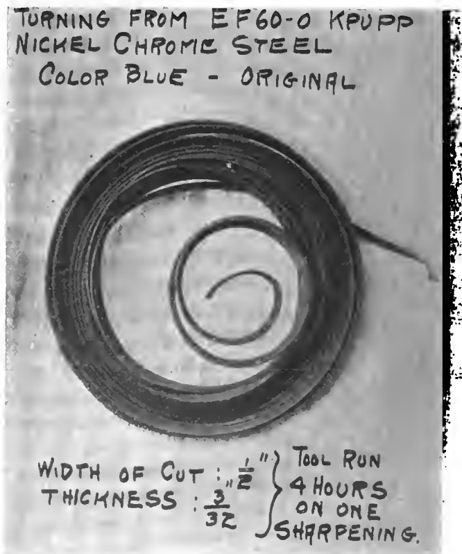
FIG. 2.—Another specimen showing capacity of heavy lathe on alloy steel.
